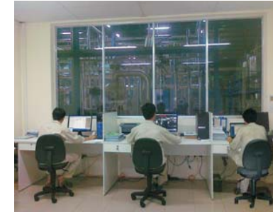
SPD production office, fully equipped with Scada software to control each step of the process.
