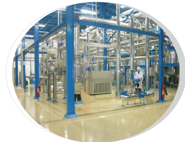
Molecular Distillation manufacturing production line to produce highly purified Omega-3 fatty acids
