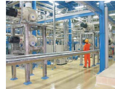
Short path distillation super High vacuum system 0.0001 mbar
