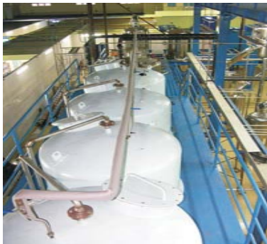
Enzyme immobilization reactor units
