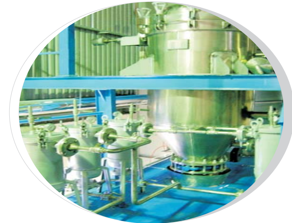
Leaf filter, bags filter and tubes filter in RBD line
